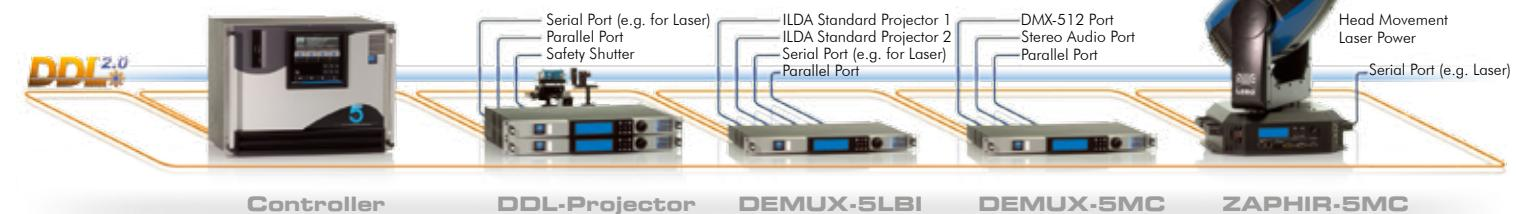
The new DDL-2® protocol allows the remote administration of all devices by the controller. Error retrieval, the detection of cabling problems and last-minute configuration changes are a matter of a few mouse clicks. DDL-2® converters provide remote ports to distribute control signals anywhere. Having to deal with just one optical cable even for multimedia shows, shortens setup times and increases the overall reliability.
